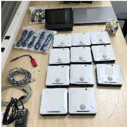
FIGURE 3. A photograph of the prototype sensor units and touchscreen gateway prior to installation. Each sensor has dimensions of 4"x4"x2". Image Credit: Amanda Kirkeby, NREL
